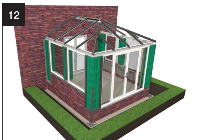
Fit and seal windows / doors against clips
