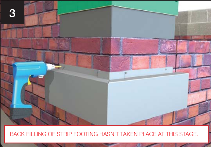
Position plinth against brickwork (to suit ground conditions). Mark through holes in plinth and then drill and plug wall. Screw plinth to wall.
