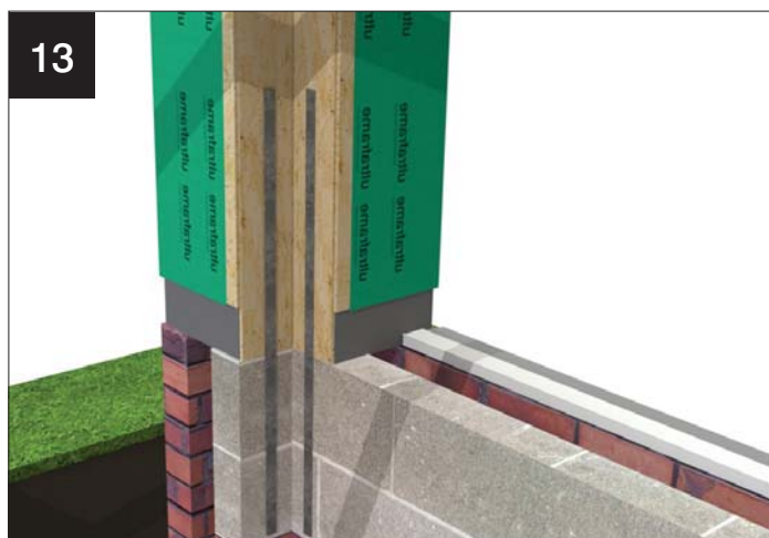
13 LARGE 90° CORNER Fasten straps down inside of walls of large 90° corner column
