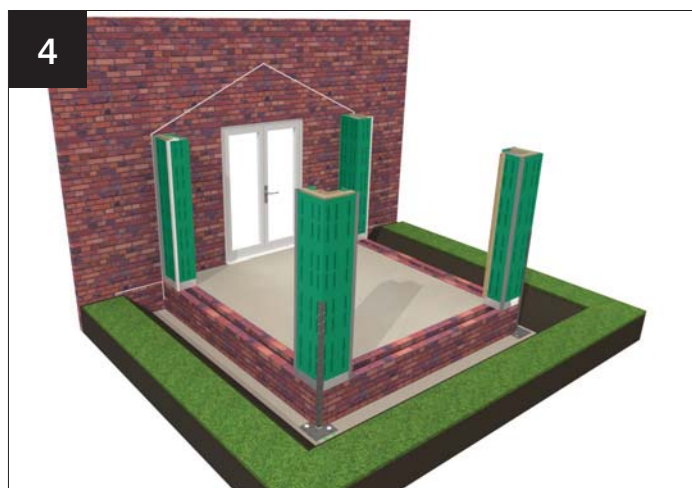
Fit abutment columns
