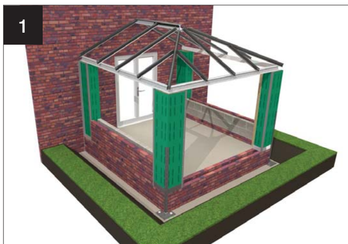
Fit windows between columns
