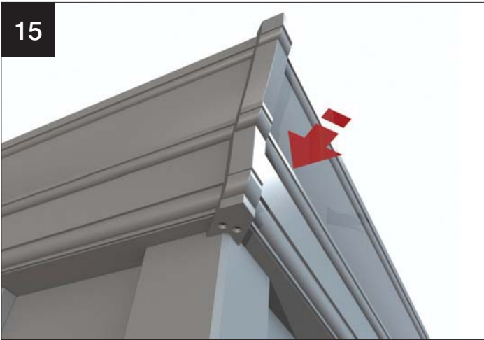
Fit Cornice corners (LRP021)
