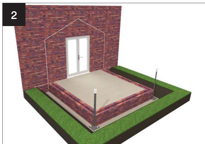
Complete base to slab level
