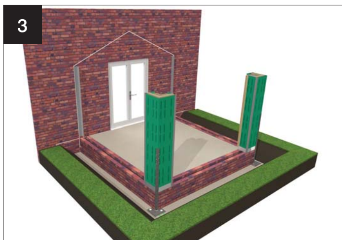
Fit corner columns
