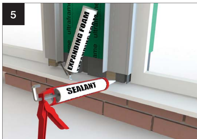
Weatherseal any joints/gaps under column and between windows/doors and columns. Use foam and/or appropriate sealant.
