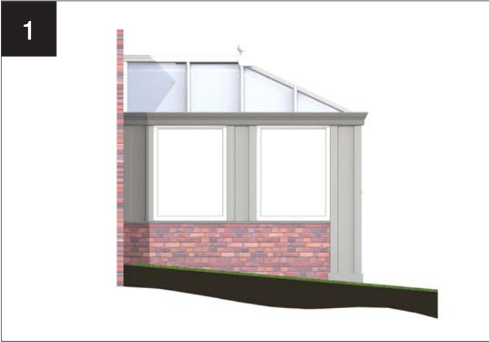
Typical build with sloping ground conditions.
