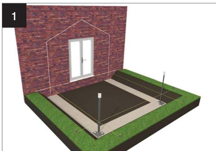
Fix brickwork set out posts to footings, align to stringline
